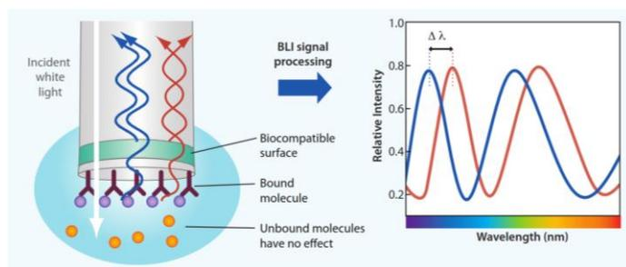
**Figure 2:** Schematic representation of a biolayer interferometry tool. Incident white light through a fiber optic cable is reflected back into the fiber optic cable from an embedded reference layer and from the biolayer attached to the end of the fiber optic cable. Peaks in the visible spectrum from each reflected wave are shifted as the analyte binds in real-time. The wavelength shift is translated to a sensorgram. From Reference 8.
