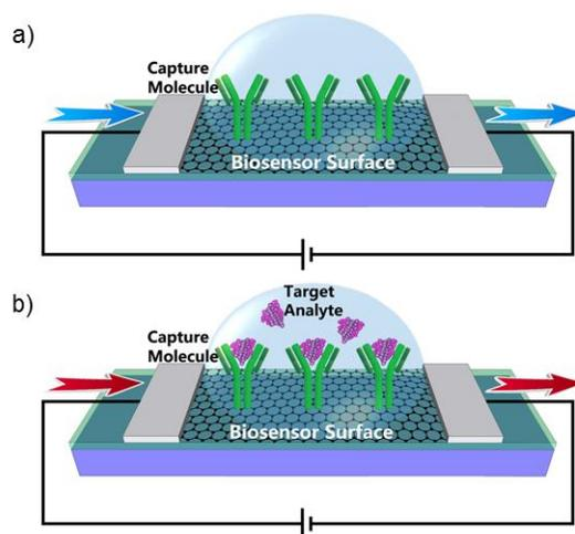
**Figure 5:** An illustration of FEB. The electrical current through a nanomaterial cell is altered when an analyte binds to its corresponding target at the sensor surface. The magnitude of the shifts in electrical properties directly correlate to the concentration of bound analyte and can be measured accurately in real-time.
