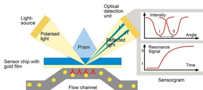
**Figure 1:** Schematic representation of a surface plasmon resonance tool. Polarized laser light is incident on a gold film which translates to an evanescent wave in the gold. The precise critical angle at which the light becomes redirected into the film is dependent on the biology on the sensor chip. The measured shift in the critical angle is recorded in real-time and translated into a sensorgram. From Reference 6.
