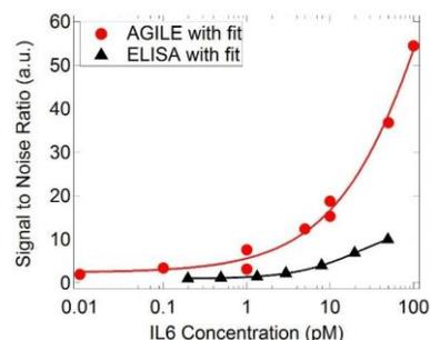
**Figure 3.** SNR data comparison of detection of recombinant IL6 using anti-IL6 monoclonal antibody with ELISA versus AGILE R100 I-Response data.
