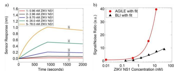
**Figure 4.** (a) Sensorgrams of anti-Zika NS1 in response to various concentrations of ZIKV NS1 on a BLI system. The LLOD is 1.4 nM. (b) SNR versus ZIKV NS1 concentration on FEB (I-Response) and BLI systems.
