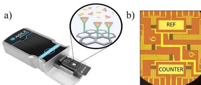
**Figure 1.** a) AGILE R100 System and illustration depicting binding of immobilized capture molecules to free-floating analyte. Image reprinted with permission from Nanomedical Diagnostics. b) Optical microscope image of sensor surface composed of graphene channels, Pt source/drain contacts, and Pt reference and counter electrodes.
