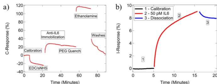
**Figure 2.** (a) C-Response throughout anti-IL6 immobilization and quenching on graphene biosensor chip. (b) Sensing and dissociation of 50 pM IL6 from immobilized anti-IL6.
