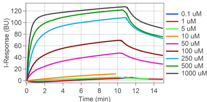
Overlay plot displays full kinetic characterization using COOH Agile biosensors. A concentration series of small molecule SPD304 is measured against immobilized TNF $\alpha$ , a cell signaling protein used as a therapeutic target. These curves show the concentration dependence of the biomolecular interaction, and the evaluation software provides  $k_{on}$ ,  $k_{off}$ , and  $K_D$ .
