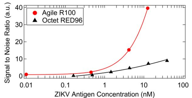
The Agile R100 measurement generated kinetic binding data comparable to that gathered on the more costly and laborious Octet RED96. On both platforms, association of ZIKV NS1 to immobilized anti-Zika NS1 was quantified using the Hill-Langmuir model of saturable kinetic binding. The resulting association rates ( $k_a$ ) were  $2.97 \times 10^4$  Ms<sup>-1</sup> on the Octet RED96 and  $9.27 \times 10^4$  Ms<sup>-1</sup> on Agile R100. These association rates agree within error.
