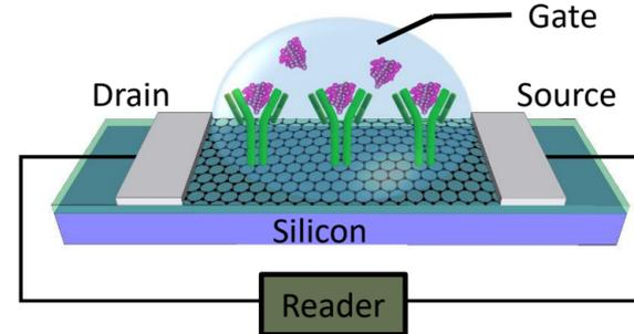
Field Effect Biosensing is a breakthrough label-free technology for measuring biomolecular interactions. It is an electrical technique that measures the current across a graphene biosensor surface functionalized with immobilized biomolecular targets. Any interaction or binding that occurs on the surface causes a change in conductance of the biosensor. FEB is a **unique orthogonal technology to optical and labeled systems** that can be used via the Agile R100 system.
